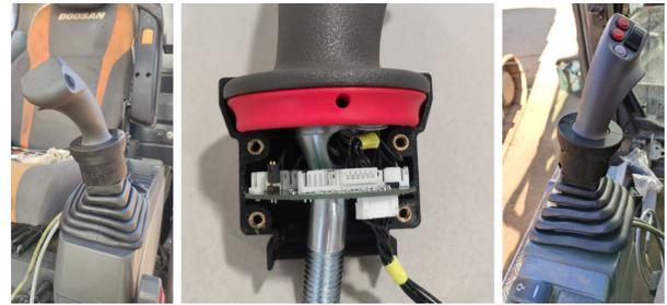
FIGURE 13. Installation of the joystick communication module on a harvester.
