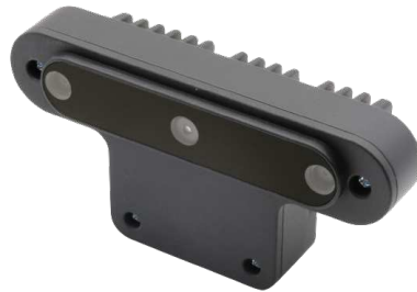
Figure 1. OAK-D sensing device accommodates an embedded inertial measurement sensor and three cameras: a monochromatic stereo-vision pair and central coloured camera. This figure is from: https://docs.luxonis.com/projects/hardware/en/latest/pages/BW1098OAK.html , accessed on 26 July 2022.
